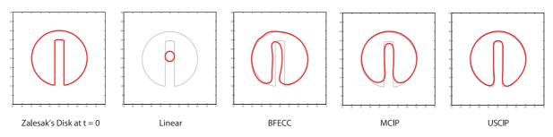
Figure 2: Zalesak's disk experiment: After one revolution on a 100×100 grid cell computational domain.
