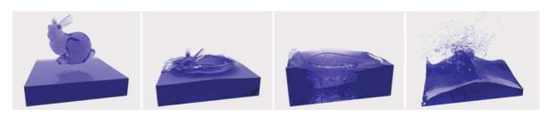
Figure 6: Simulation of a bunny-shaped water chunk dropping onto still water. The grid resolution was 150<sup>3</sup>.
