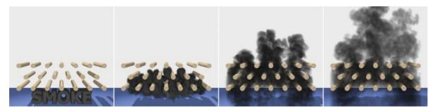
**Figure 5:** Simulation of rising smoke passing through obstacles. The grid resolution was  $160 \times 220 \times 80$ .
