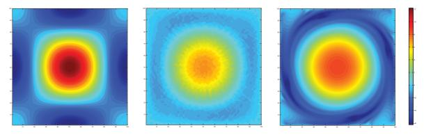
**Figure 8:** 2D Vorticity preservation test on a  $100 \times 100$  grids. The left image shows the magnitude of initial vorticity. The middle and the right images show the results of the FLIP and USCIP methods, respectively, at t = 3.0 sec. In the images, color represents the magnitude of the vorticity.
